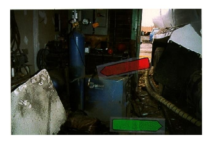
**Photograph** #7 – Shows the wire feed welder's position with respect to the tank truck. Green arrow [lower arrow] shows the overflow pipe location. Red arrow [upper arrow] shows the welding stinger used to strike the arc.
