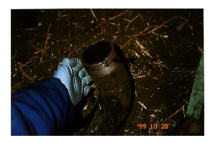
**Photograph** #5 – Shows overflow pipe elbow. Arrow shows where a welding arc had been struck.
