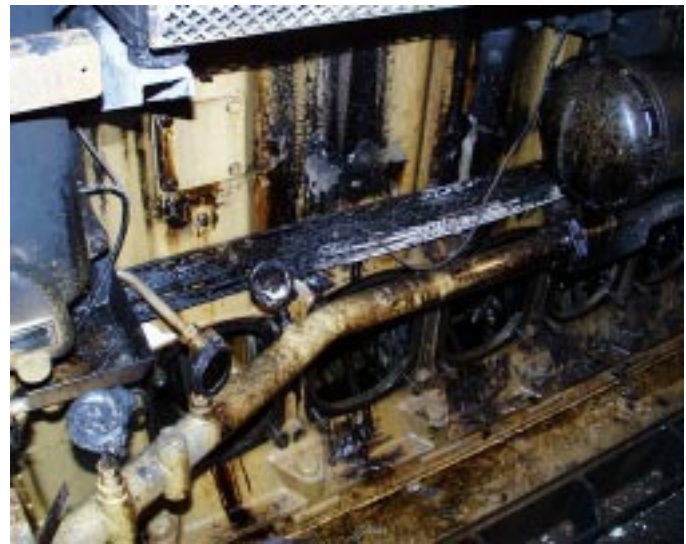
FIGURE 7 Port side of engine showing stripes of scorched paint
