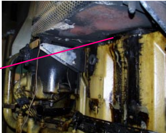
FIGURE 7 Port side of engine showing stripes of scorched paint
